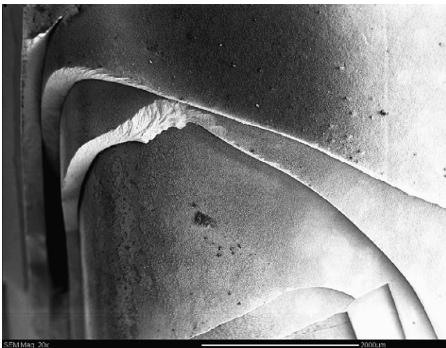
Fig. 14. Radial and axial direction of a crack propagation 22 .
